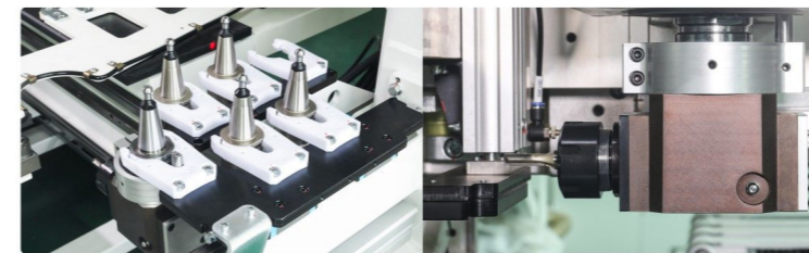
可选:六刀位自动换刀刀库和铣型角度头 Optional: ATC 6 by servo and single aggregate
